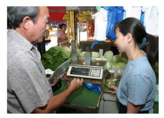
Measurement Standards inspector Wendell Murakami (I) tests a produce scale for accuracy at a market in Chinatown and explains the procedure to the vendor.
