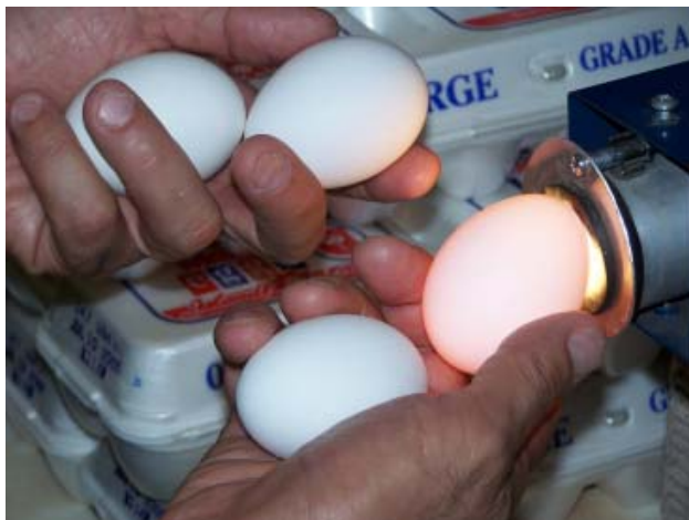
Above: Egg inspectors use a "candler" to inspect eggs for quality and grade.
