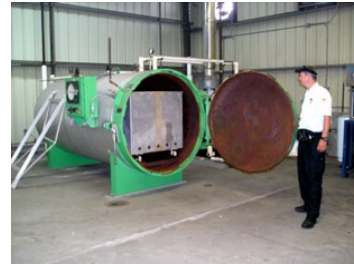
Large capacity sterilizer housed in cargo building.
