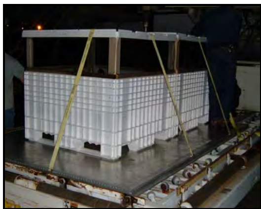
Figures 6 & 7. Figure 6 illustrates how a crate is secured to "cookie sheet" being loaded on to an aircraft. Figure 7 illustrates how the "cookie sheet" is secured to the aircraft. Photos courtesy of Lauren DuBois
