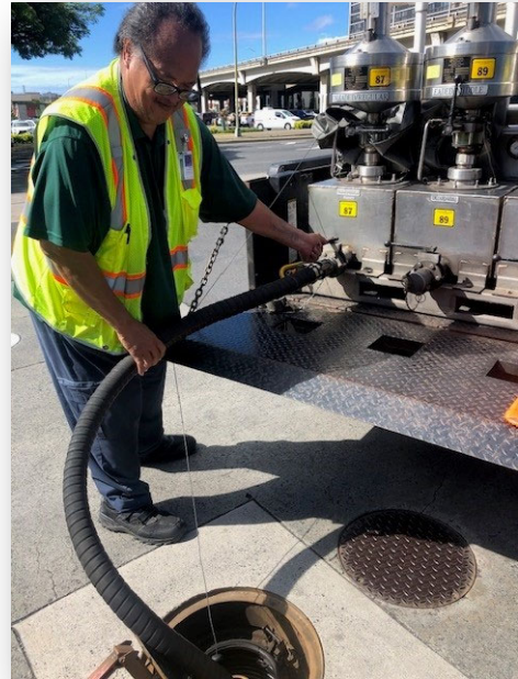
MS inspector Sione Feleunga discharging fuel to an in-ground storage tank after inspecting the gas pump meter
